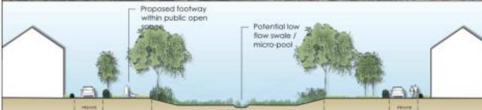
ILLUSTRATIVE LANDSCAPE SECTION C-CC 1:250 : GREEN CORRIDOR Positioning of proposed built form or landform is indicative and subject to detailed design.
